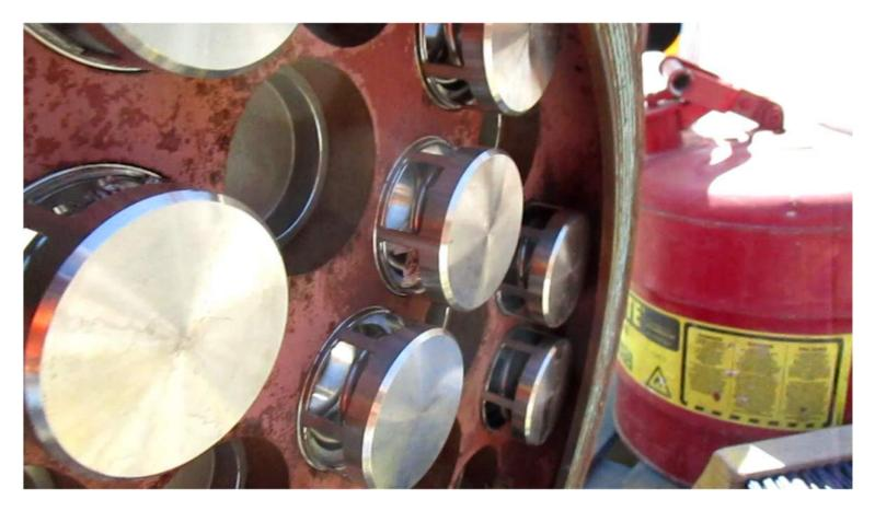
Ported cylinders are spring-actuated to deliver design flow.
