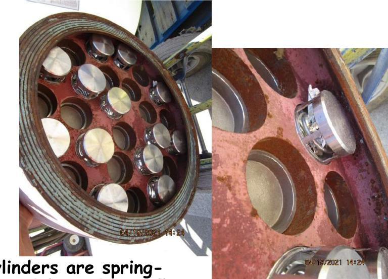
Ported cylinders are springactuated to deliver design flow.
