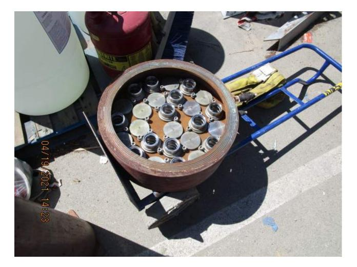
Flow limiters prevent exceeding a given maximum flow rate.
