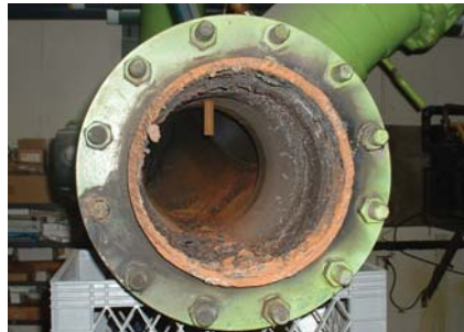
PHOTOS A and B. Both of these pipes are the same age and served the same chiller, seeing nearly identical operating hours. The one on the left is the condenser-water line (an open system), while the one on the right is the chilled-water line (a closed system). Both systems were provided with a water-treatment program by a competent contractor, with oversight by a knowledgeable owner.
