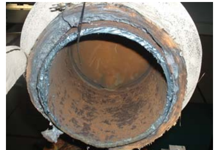
PHOTOS A and B. Both of these pipes are the same age and served the same chiller, seeing nearly identical operating hours. The one on the left is the condenser-water line (an open system), while the one on the right is the chilled-water line (a closed system). Both systems were provided with a water-treatment program by a competent contractor, with oversight by a knowledgeable owner.
