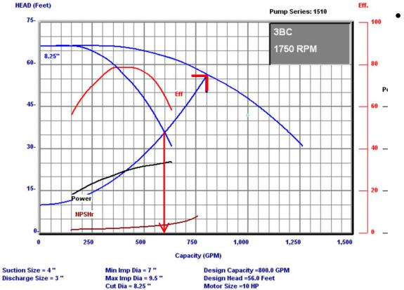
The Power and Eff. curves shown are for the cut dia. impeller.
