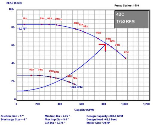
The Power and Eff. curves shown are for the cut dia. impeller.
