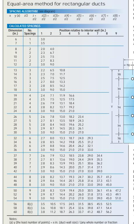
FIGURE 2. Equal-area traversal points and spacing algorithm for 6-in. square duct.
