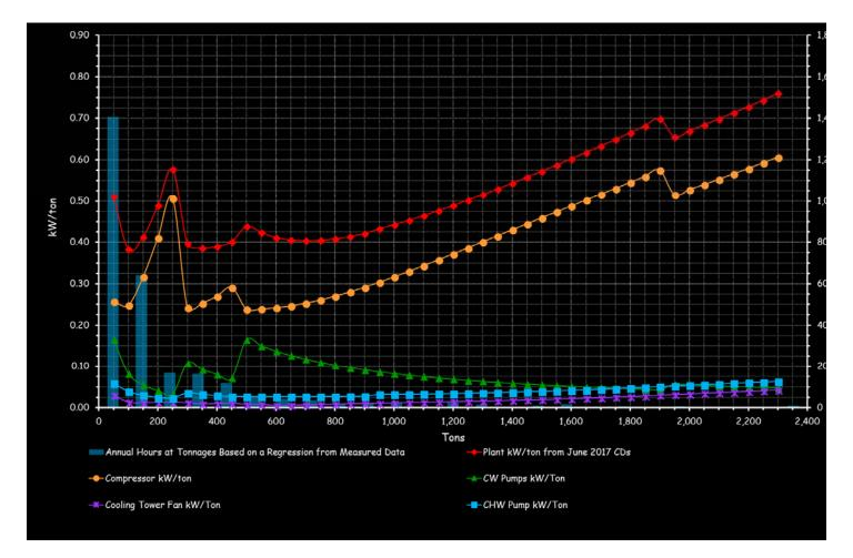
The blue bars represent the load profile for a 59 or so story high-rise up in Seattle, which is where this plant is located. I was involved because they were getting ready to upgrade their plant and I suggested the perhaps we should let the building tell us what the chiller tonnage break-down should look like and then pick the machines and develop the sequence on that basis.
