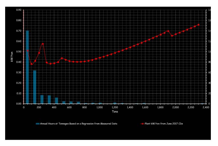
So, what we would like to do for a field based class at your hotel would be to develop this profile for your plant (the red line) and if possible, contrast it for the measured load profile for your plant (the blue bars).
