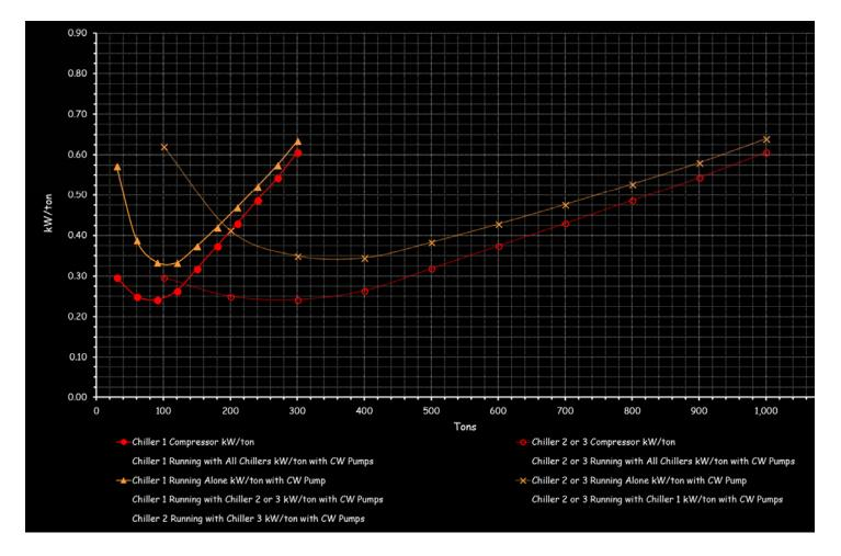
Even thought intuitively, it would seem like you would want to run the 300 ton modular chiller until it was fully loaded, it turns out that if you look at the compressor kW per ton curves for it and the larger machine, the larger machine compressor energy is actually lower than the 300 ton machine starting around 130 tons (where the 2 red lines cross). When you toss the condenser pump energy into the mix, that point shifts to about 185 - 190 tons (where the two orange lines cross above).
