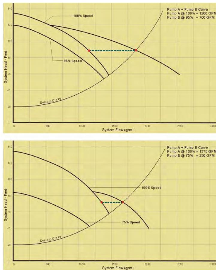
The system curve is accurate so long as nothing in the system changes. When two-way valves are incorporated into the system, the variable pressure drop created changes the system curve. This is important to understand because in a variable flow system with multiple two-way valves, there are many system curves that may represent the condition at various times.
