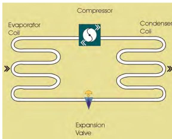
The refrigeration cycle diagram shows the relationship of these components, as does the pressure-enthalpy chart, also known as a P-H diagram. These diagrams cover the liquid-vapor regions specific to the cycle refrigerant. The following is a description of the refrigeration cycle:
