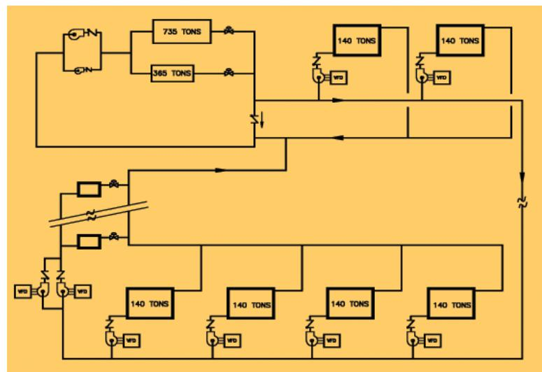
Note that a check valve has been provided in the common leg of the primary-secondary system to ensure that primary flow is always less than secondary flow. This places the primary and secondary pumps in series during transients such as cool-down (which are all but non-existent in the San Francisco climate).
