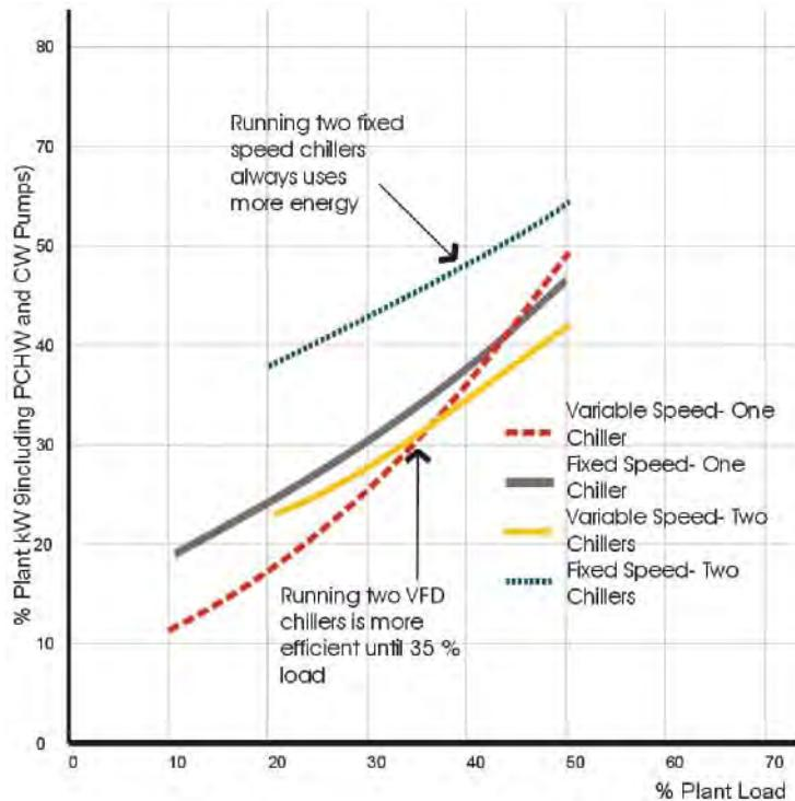
The net effect of these chiller performance characteristics, when combined with the energy usage of ancillary pumps and tower fans, is that:
