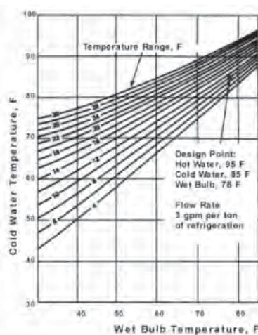
Cooling towers are relatively inexpensive when compared to the total cost of a chiller plant, and incremental increases in tower size and energy efficiency can be purchased at a very low cost. Skimping on the cooling tower is penny-wise and pound-foolish. Every effort should be made to optimize the selection of the tower. Matching larger fill volumes with lower fan capacities is a very good investment.
