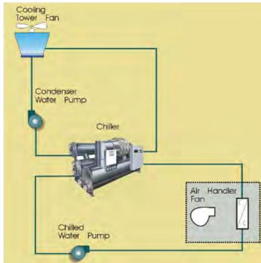
Nevertheless, it is possible to partially optimize the chiller plant with a reasonable engineering effort. The key is to break the chiller plant into subsystems and then optimize within those subsystems. The plant will not be completely optimized due to the complex interaction between subsystems, but the result should be close to optimum.
