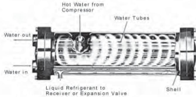
High water velocity is recommended in the condenser tubes as it increases the heat transfer effectiveness and reduces fouling. Water velocities of at least 3 feet per second and a maximum of 12 feet per second are recommended. A minimum flow is needed to maintain flows above the laminar range and the maximum flow protects the tubes from erosion and keeps pressure drops to a minimum. In the HVAC industry, water pressure drops through the condenser are seldom over 25 to 30 feet of water column.
