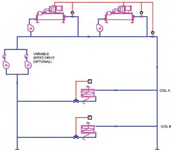
Another issue in primary/secondary piping is the size of the common piping (bypass pipe). In a multiple chiller system that is properly controlled, the maximum flow in the bypass should not exceed 110% to 115% of the flow from one chiller. However, in most cases the bypass line should be the same size as the supply and return header. There are two reasons for this:
