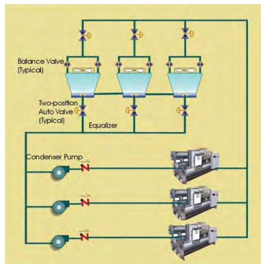
In a multiple chiller arrangement a standby pump (Figure 4-24) is sometimes provided for redundancy. In this arrangement, adding the standby pump is cumbersome and requires a number of added valves.
