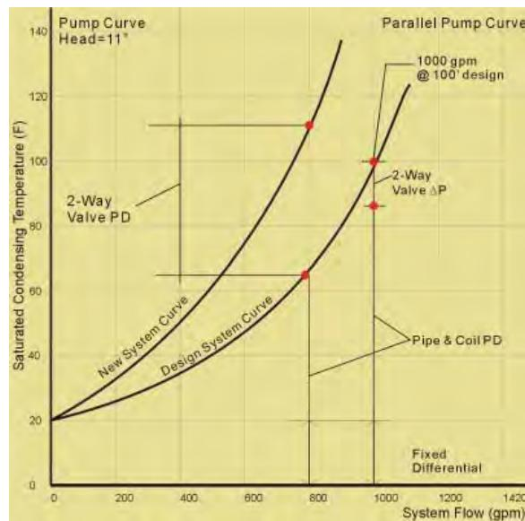
Depending if the active loads in a piping system are near to or far from the pump, a range of system curves best describes the conditions that may occur at any given time. As the flow decreases, the velocities of the water in the pipe can develop laminar flow or a mixed laminar-turbulent flow. This has the effect of decreasing the exponent in the system curve equation above and is another reason to expect a range of system curves in an operating system.
