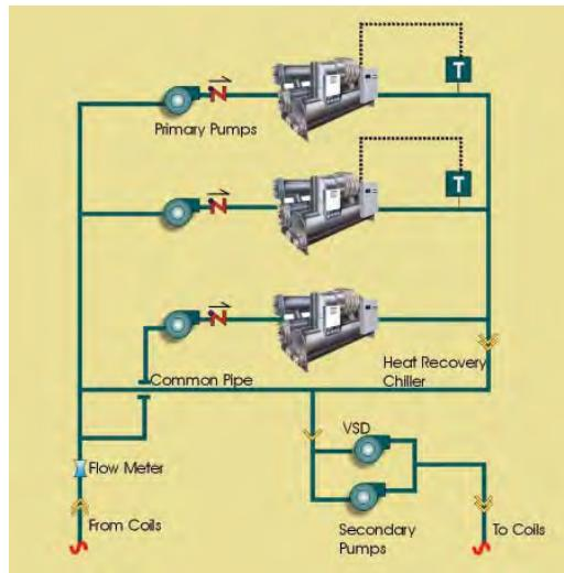
Figure 4-21 shows a configuration for a heat recovery machine that essentially puts the machine in series with the remaining chillers in the plant. Warm return water is pumped to the chiller then back into the return, thereby precooling the inlet water to the other chillers. The heat recovery machine can remove as much or as little heat as is needed for the heating load.
