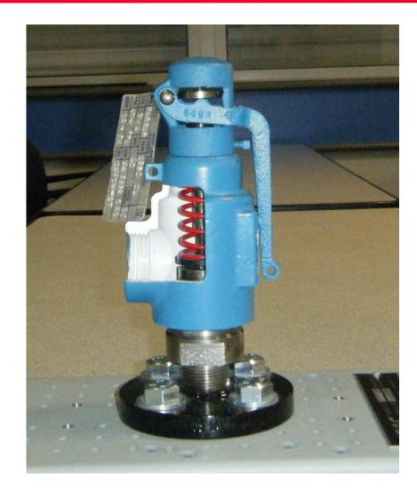
Disk lifts against a spring to allow flow up to a specified pressure
