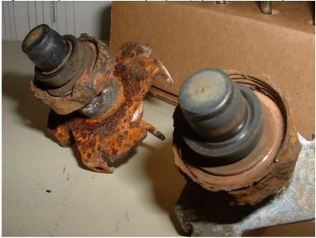
d. The valve plugs on the original hot water valves were rubber, which over the years has cracked and eroded away, resulting in significant leak-by when the valve is closed. In addition to compromising the cooling capability of the fan coil unit, the leak-by imposes a simultaneous heating and cooling load on the central plant.
