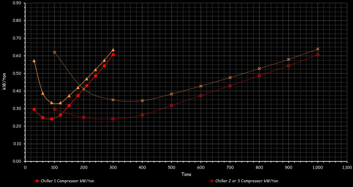
Chiller 1 Running with All Chillers kW/ton with CW Pumps ← Chiller 1 Running Alone kW/ton with CW Pump
