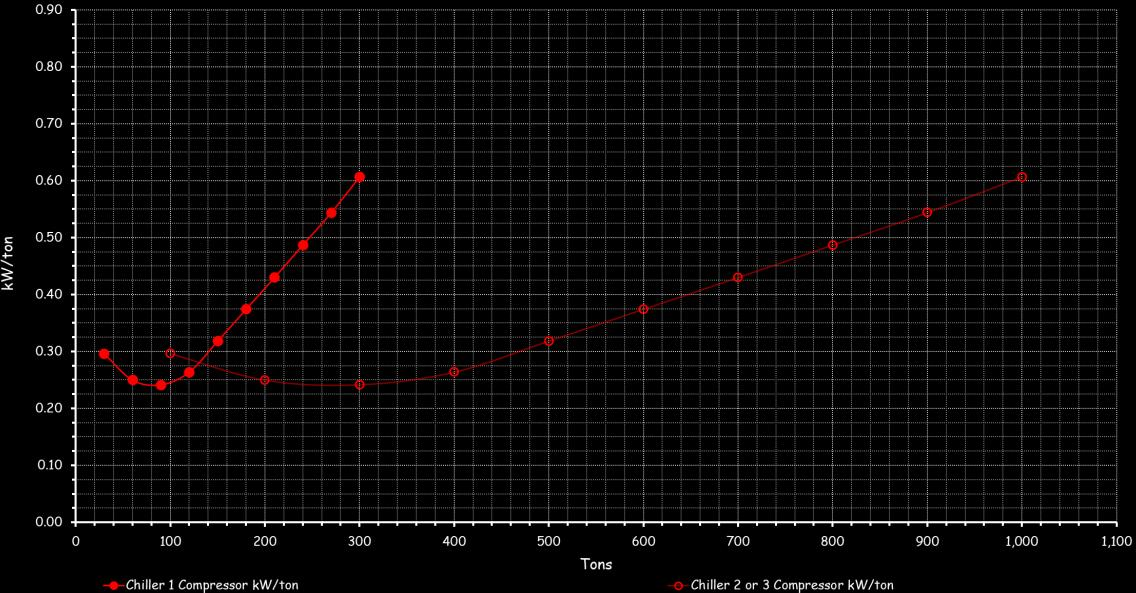
Chiller 1 Running with All Chillers kW/ton with CW Pumps
